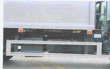
Wastewater collection tank
